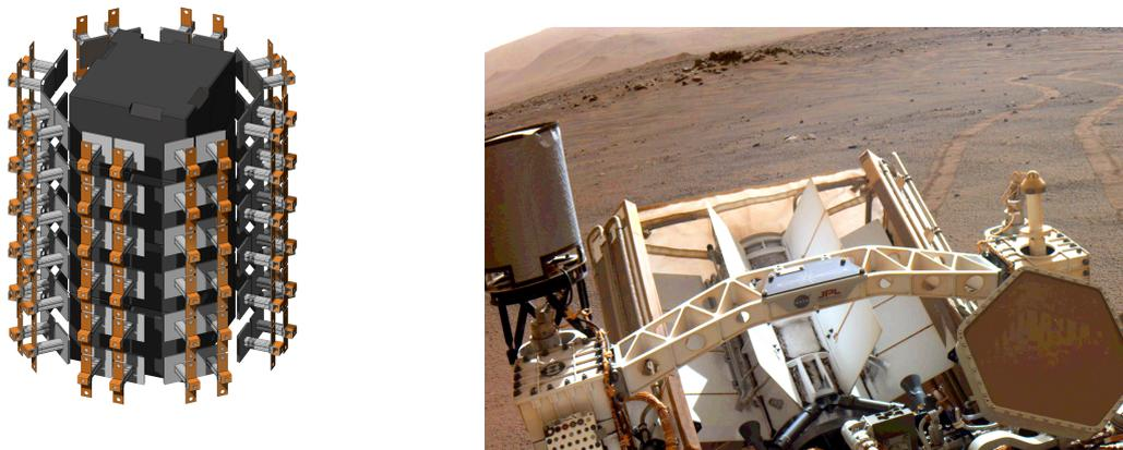
Figure 1: A stack of 3 GPHS Bricks surrounded by hot shoes and thermoelectric legs (left) and the Perseverance mission RTG with exposed radiative fins [2] (right)
