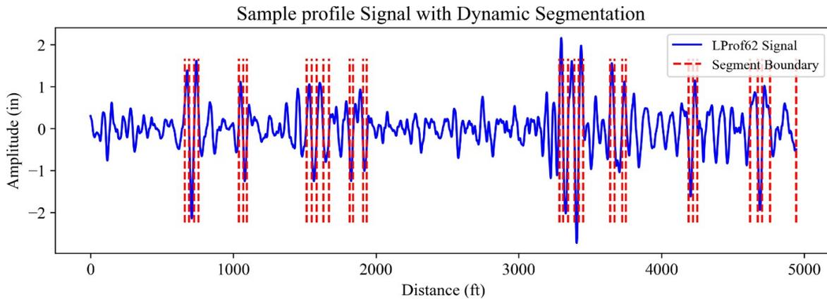
Figure 6: Dynamic (variable-length) Segmentation
