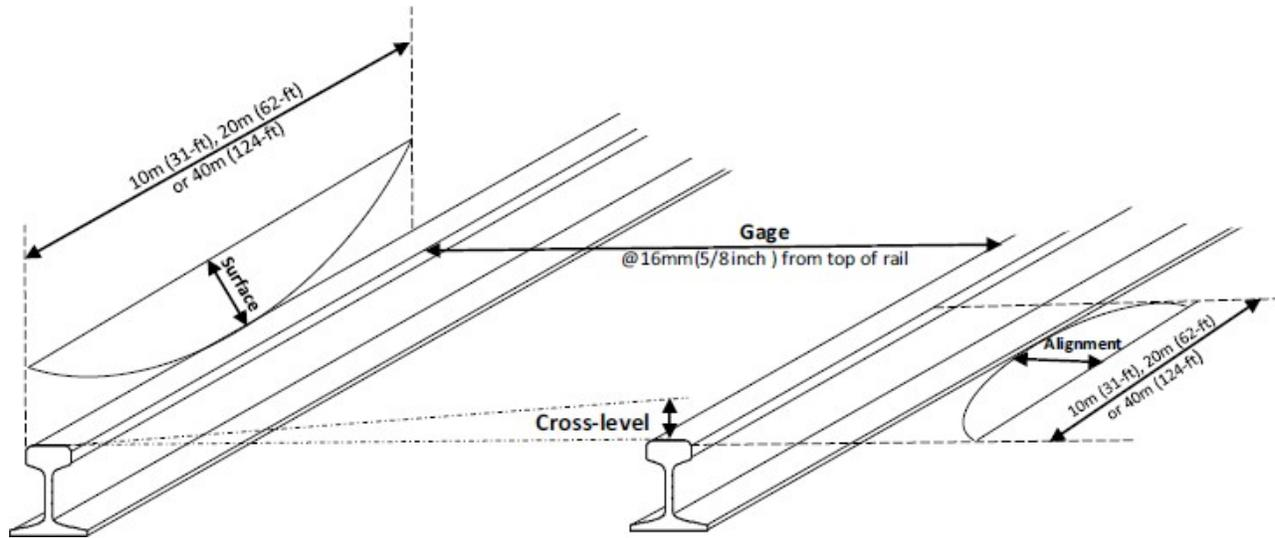
Figure 1: Schematic diagram of track geometry parameters (Lasisi & Attoh-Okine, 2019)
